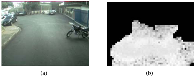
Fig. 6. (a) is a color image. (b) is results from a classification sample from our system. Black represents non-road class, white represents road class and the gray represents the intermediate values.
